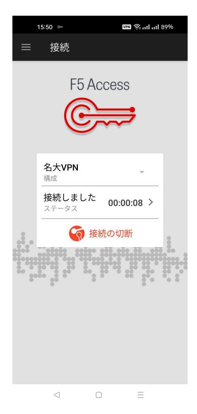
Once "Connected" is displayed, the VPN connection is established. To disconnect the VPN connection, press "Disconnect".
